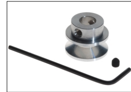
Pulley. 2mm I.D. (16mm dia. x 13.6mm) (Aluminium). 6g Part No: 918D3
