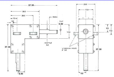
This unit has steel gears and shafts running in ballraces and scintered bronze bearings, 1 ball race and sintered bearing per shaft. The former act also as thrust races protecting the bevel gears from external pressures of varying loads. The housing mouldings are 30% glass filled nylon for strength and have four pre-drilled mounting holes. Key flats are provided on both shafts.
